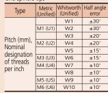
Note) This chart indicates the difference between the angle made by anvil's contact faces and spindle's axes and the half angle with error  $\alpha$ . Metric/Unified  $\theta = 60^{\circ}$  Whitworth  $\theta = 55^{\circ}$
